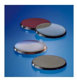
Figure 2: Fused bead samples with different iron concentrations
