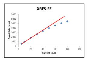
Figure 4: Linearity of the scintillation counter.
