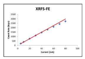
Figure 3: Linearity of the flow counter.
