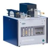
Bruker's G4 PHOENIX was developed for the fast and easy determination of diffusible hydrogen in welds and other sample matrices using the carrier gas hot extraction method.
