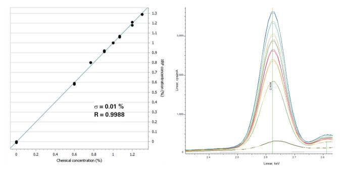
Fig. 7 Calibration for NaCl in saline solution. a) Calibration curve for given vs. measured concentrations.  $\sigma$  is the standard deviation in weight percent, R<sup>2</sup> the squared correlation coefficient. b) Spectra of the calibration standards.
