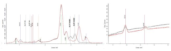
Fig. 4 Spectra of KCl and NaCl from different providers. The different amounts of Br are well resolved.
