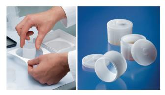
Fig. 8 Preparation of sample cups for liquid and loose powder samples.
