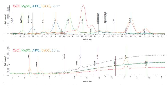
Fig. 5 Spectra of various salts used in the pharmaceutical industry. The lower part shows someof the common contaminants found in these substances.
