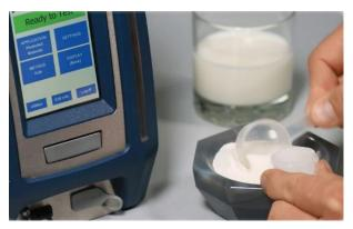
Portable XRF is used to measure mineral nutrients in powdered milk.
