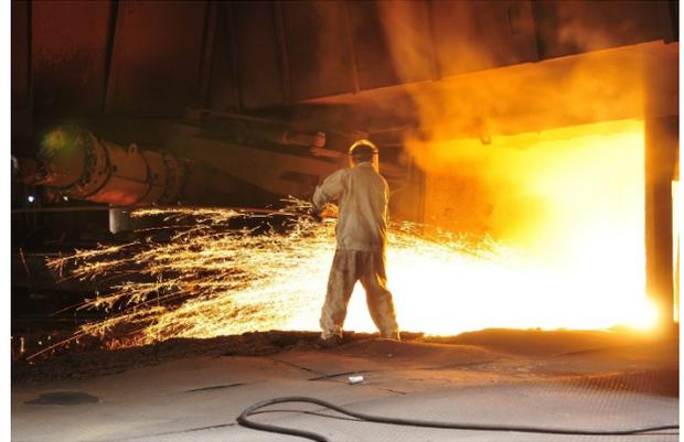
*Steel blast furnace taphole spewing molten iron.*
