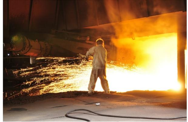
*Steel blast furnace taphole spewing molten iron.*
