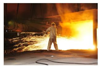
Steel blast furnace taphole spewing molten iron.
