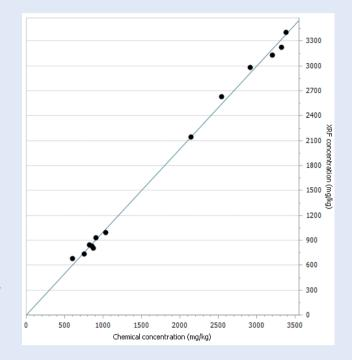
Fig. 1: Calibration curve for Na (KA1) measured in milk protein by using the S2 PUMA (EDXRF); sample preparation: pressed pellets.
