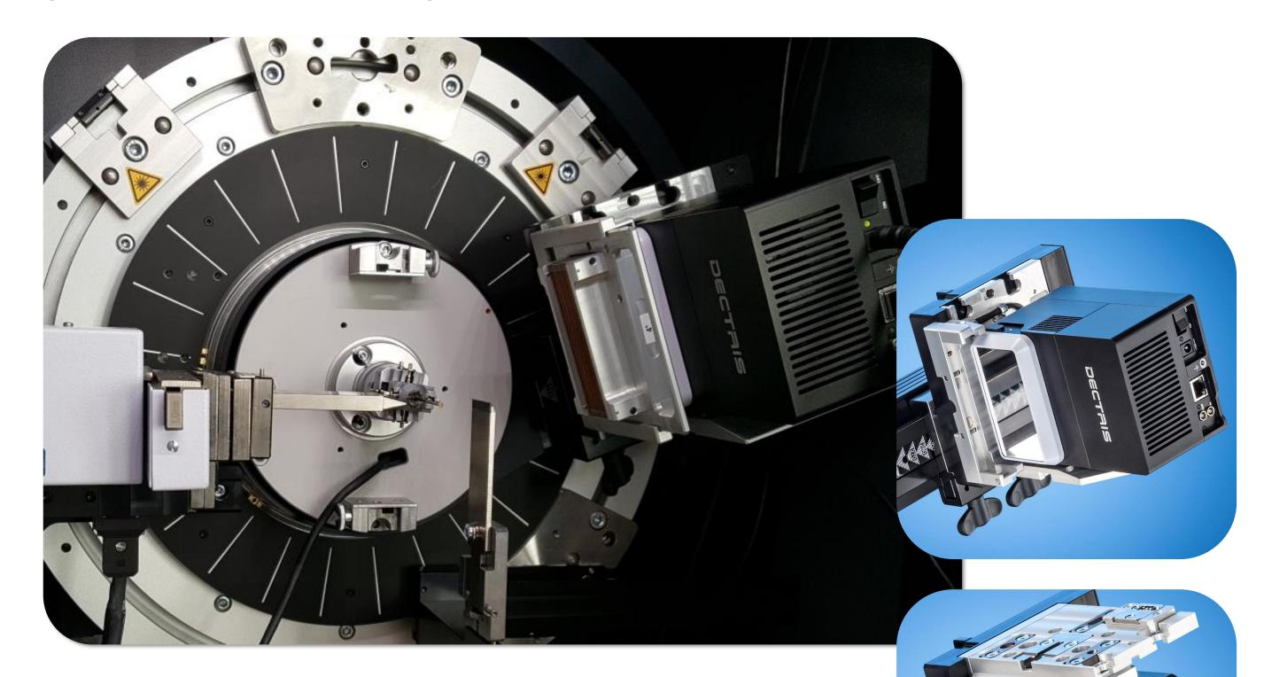
(Above) D8 ADVANCE diffractometer with molybdenum source, focusing Goebel mirror, capillary stage, and EIGER2 R 500K
