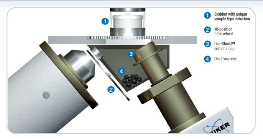
SampleCare<sup>™</sup>: A unique, multi-layer system to protect vital system components
