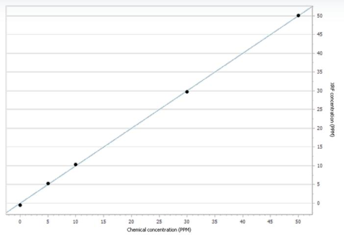
• Example of P calibration curve in the range of 0 to 50 ppm P
