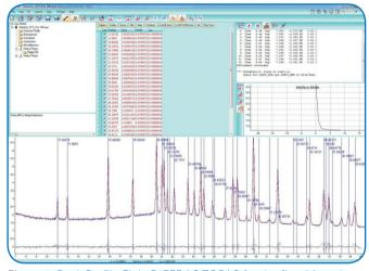
Figure 4 Peak Profile Fit in DIFFRAC.TOPAS for the first 30 peaks. The peak shapes were constrained to have the same FWHM and Lorentzian component parameter, Lor.
