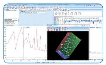
Figure 10 After refining three torsion angles the Rwp values drops significantly to approx. 12%. The only obvious misfit is the background at higher angles.
