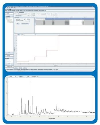
Figure 2 Variable Count time scheme, as defined in the Wizard plugin of the measurement software and corresponding data set shown in the results manager. The resulting steps in the data are automatically scaled in the DIFFREC.EVA or DIFFRAC.TOPAS software packages.
