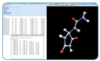
Figure 7 Rigid body editor in DIFFRAC.TOPAS. The point\_for\_site notation is useful to enter xyz coordinates. The "first Guess Z-matrix" option will convert to a z-matrix notation that can be parameterized and refined to make the model structure less rigid.
