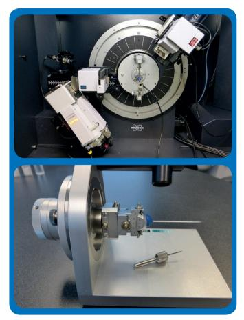
Figure 1 D8 ADVANCE configuration used for data collection with primary beam monochromator, capillary stage and LYNXEYE XE detector. Low absorption glass capillaries with 1 mm diameter were used, filled with Allantoin and sealed off with a lighter. The capillary was mounted on the goniometer head using modelling clay for support and centered in the beam using the alignment microscope to avoid any wobbling.
