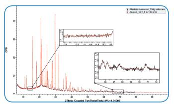
Figure 3 Comparison of scans with constant time/step (black) and variable count time (red) scheme from Figure 2. The improvement in counting statistics is evident at higher angles.
