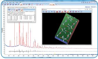
Figure 11 Result with Rwp =4.4% after refining only three torsion angles and the background function.
