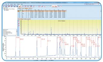
Figure 5 Results of the LSI Indexing algorithm using DIFFRAC.TOPAS. The solutions tab displays a list of possible unit cells and a graphical representation of the Goodness of Fit (GOF) versus the cell volume. The smallest unit cell that explains all observed peaks without any additional calculated peak positions (displayed as dashed lines) is likely the correct solution.
