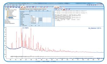
Figure 6 Pawley Fit of Allantoin. The amorphous halo from the glass capillary was fitted with a single broad peak. After checking for a sensible background shape, especially at high angles, all refinable parameters were fixed and the resulting project exported to an INP file, which serves as the starting point for the structure solution in the Launch mode of DIFFRAC.TOPAS.
