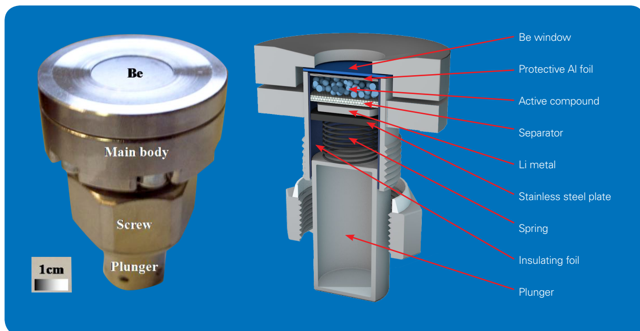
Fig. 1: Battery cell basic design
