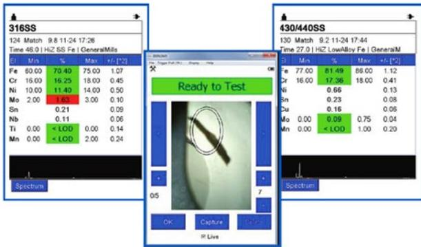
*New HXRF instruments can pinpoint the sample spot with an integrated camera and small sample spot collimator for precise analysis of miniature components.*
