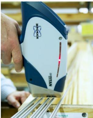
*Bruker's Handheld XRFs are used throughout industry for QA/QC, alloy identification, and failure analysis of incoming and in-use standard metals and alloys.*
