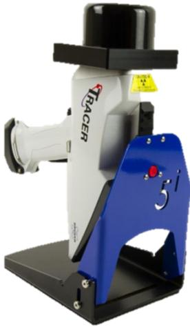
*Optimal HHXRF presentation for some new materials involves placing powders in an XRF sample cup with thin XRF film and using a desktop stand with the nose up for reproducible testing.*
