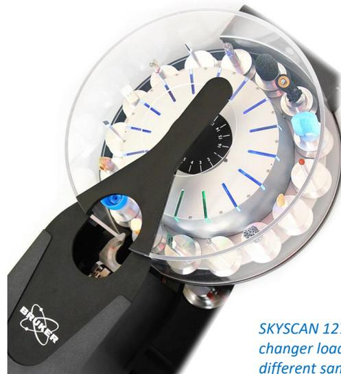
*SKYSCAN 1272 sample changer loaded with different samples.*
