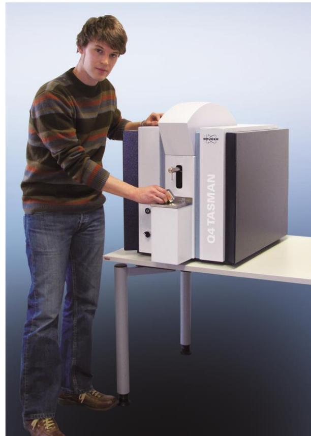
*Q4 TASMAN optical emission spectrometer for metals analysis*
