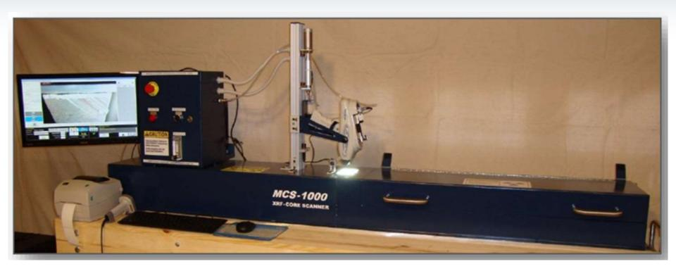
Max 4 inch core in 3 feet (1 m) standard segments TRACER IV SD system with He purge for Na-U elemental range
