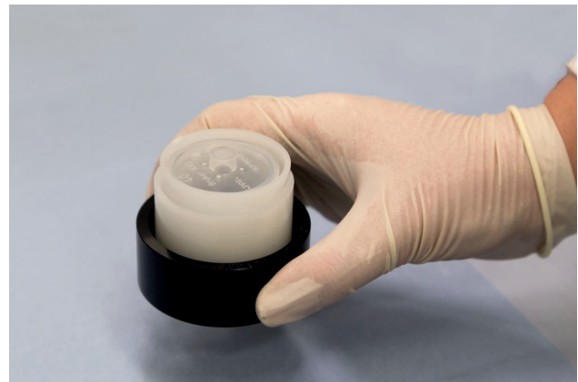
Figure 3: Liquid cup (Ø 40 mm) in SampleCare cup (Ø 51 mm). The liquid cup preparation tool can also be used to transport the samples from lab bench to measurement chamber.
