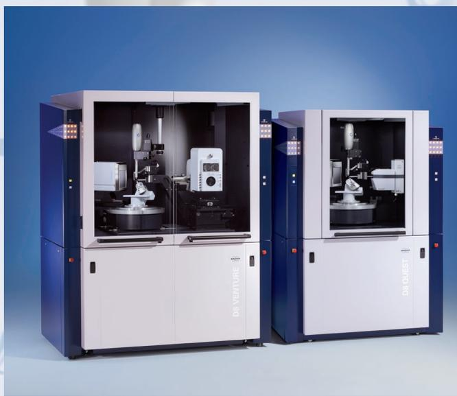
The new PHOTON III detectors are available in various sizes and are integrated with the D8 VENTURE and D8 QUEST X-ray crystallography solutions.
