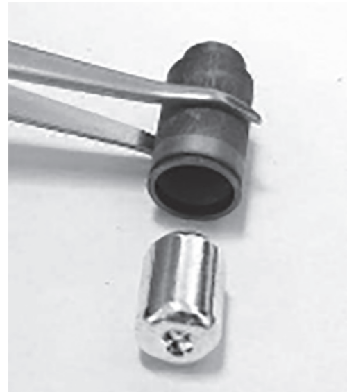
Figure 7 The sample can be easily removed from the reusable crucible
