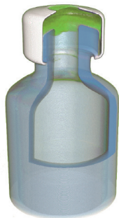
Volume render of a glass vial with rubber seal and aluminum cap Scanned with the SKYSCAN 1275
