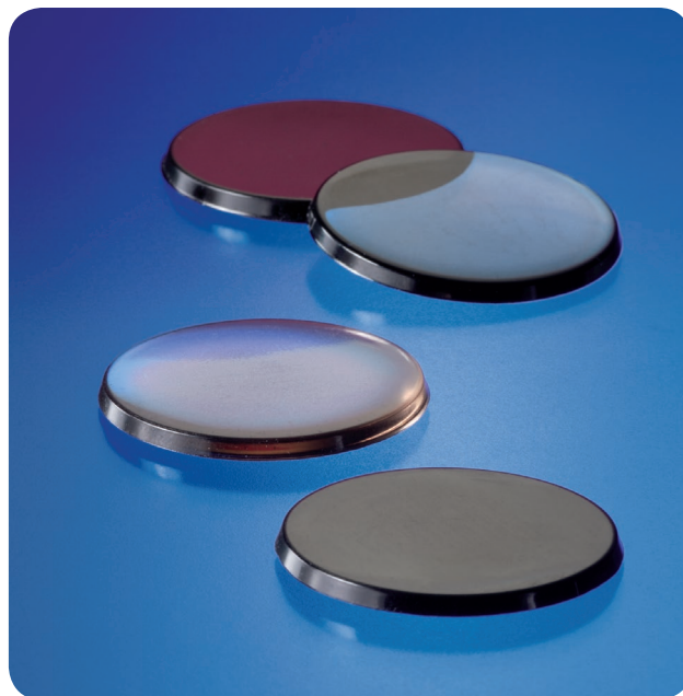
Fig. 2: Samples prepared as fused beads
