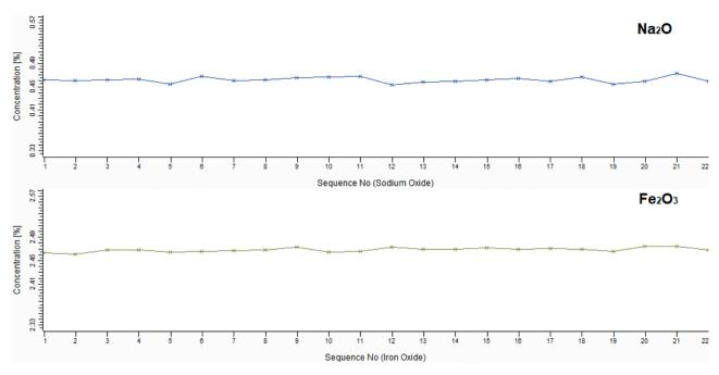
Figure 3: Repeatability for Na and Fe (t = 21 hours). Plots produced by Bruker's SpectraElements software.
