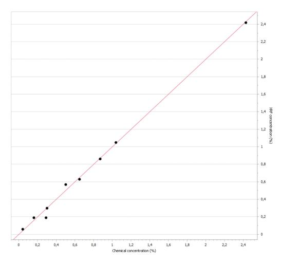
Figure 2: Calibration curve for Fe. Plot produced by Bruker's SpectraElements software.
