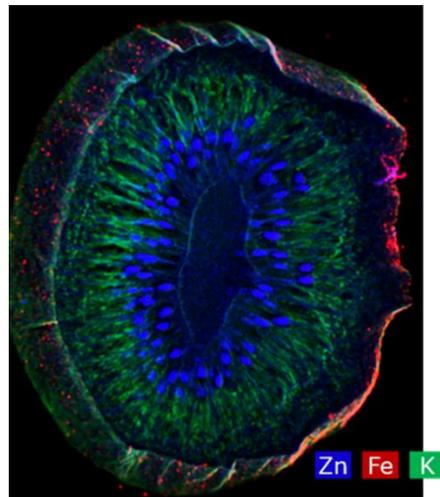
*Micro XRF elemental distribution map of zinc (Zn), iron (Fe), and potassium (K) in a kiwi slice.*
