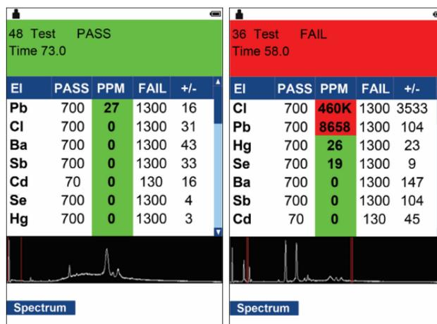
Portable XRF identifies products that pass or fail safety with preset thresholds.
