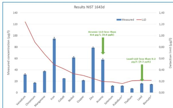
TXRF can identify heavy metals at levels below 1 ppb.
