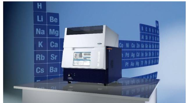
*Modern Lab XRF spectrometers are equipped with an XY-Autochanger, allowing high throughput at production facilities.*
