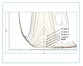
Figure 5: Overlaid sulfur signals in gasoline starting with a blank signal, followed here by 5, 10, 15 and 25 ppm S. The integration range is shown in orange.
