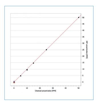
Figure 4: Calibration curve for sulfur in gasoline for the low concentration range between 0 to 50 ppm  $\mbox{\ensuremath{S}}$
