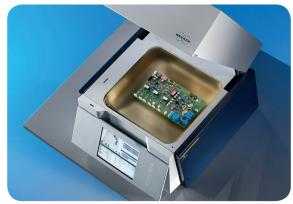
Figure 1: The S2 PUMA – the all-round EDXRF instrument
