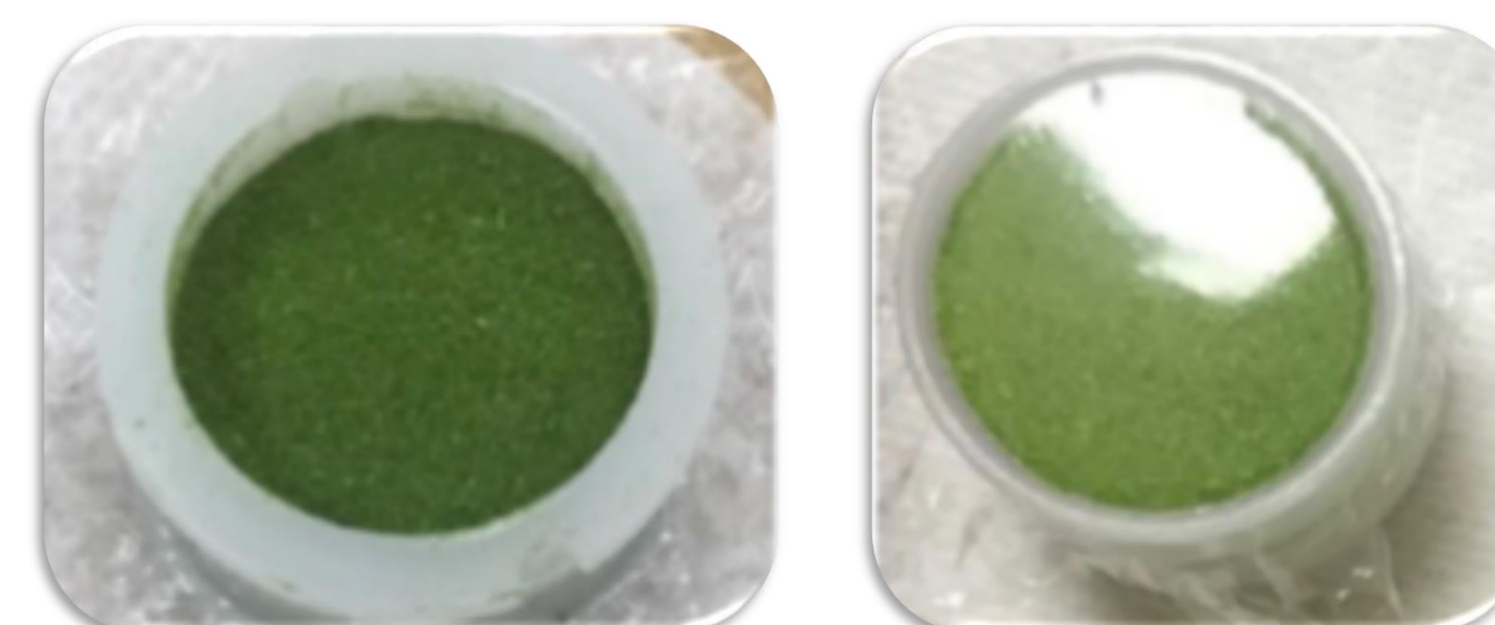
Figure 1a and 1b. Spinach leaves crushed and prepped for analysis; packed in cup
