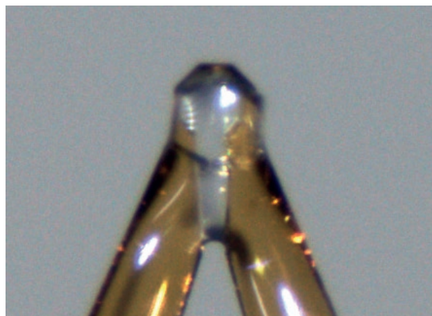
Figure 2: D8 VENTURE video image of the 20 \times 55 \times 65 \text{ \mu m}^3 lysozyme crystal.
