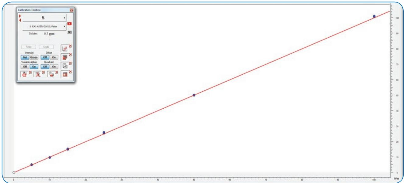
Figure 2: Calibration curve for sulfur in fuels according to ASTM D 2622 covering 0 – 100 ppm
