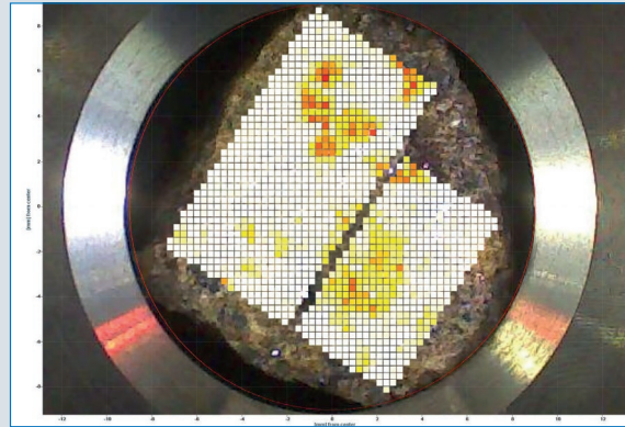
Figure 6: Element map of titanium analyzed with the S8 TIGER Series 2
