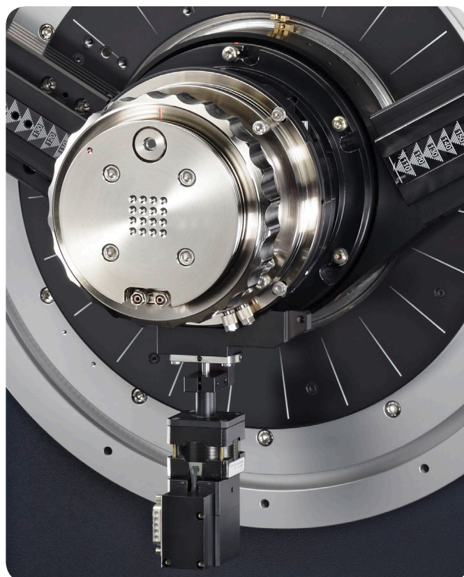
MTC-HIGHTEMP chamber with motorized height alignment stage
