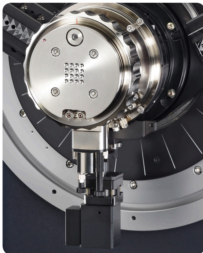
MTC-HIGHTEMP+ chamber with motorized height alignment stage
