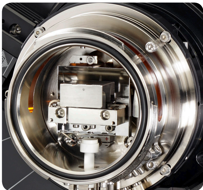
MTC-FURNACE interior with the corundum sample spinner moved out of the way
