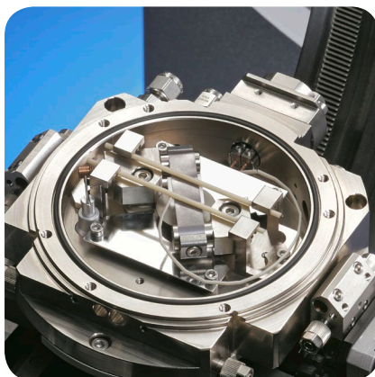
TC-DOME configured for thin film samples
