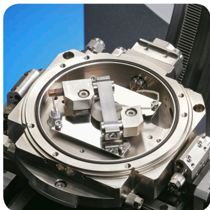
TC-DOME configured for powder samples
