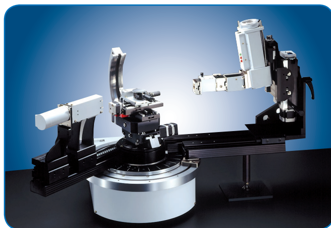
Figure 2: The D8 DISCOVER Ultra-GID, which can be configured for coplanar (left) or non-coplanar („in-plane“) measurements.
