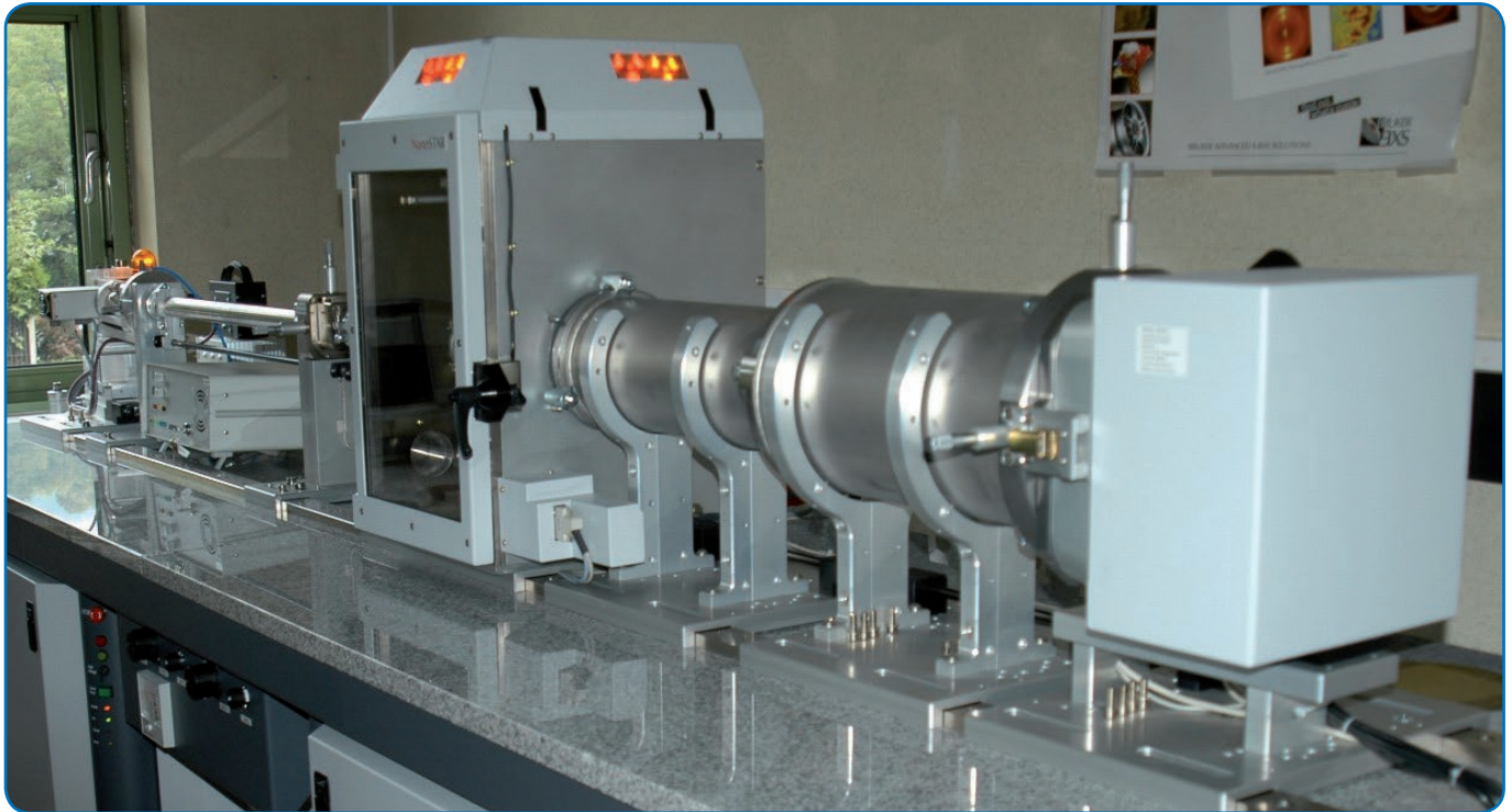
Figure 1: NANOSTAR-U with I_{\mu S} (left), extended sample chamber with WAXS Image Plate detector (center), and a 20 \times 20 \text{ cm}^2 active area VÅNTEC-2000 (right).
