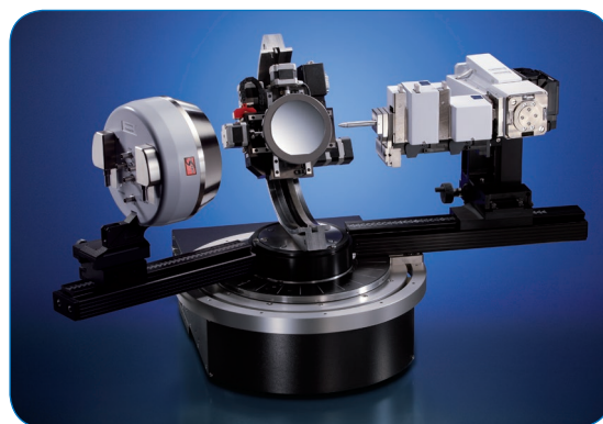
Fig. 1: Centric Eulerian cradle mounted to horizontal D8 DISCOVER with VANTEC-500 area detector
