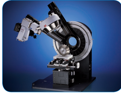
Fig. 3. UMC 150 stage for residual stress analysis
