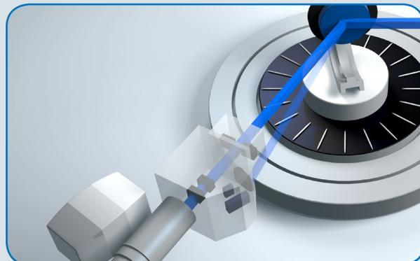
Fig. 6b. High-intensity beam path for GID and XRR on very thin films
