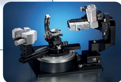
Non-coplanar diffraction gives direct access to the in-plane lattice parameters, in-plane crystallite size and in-plane preferred orientation.
