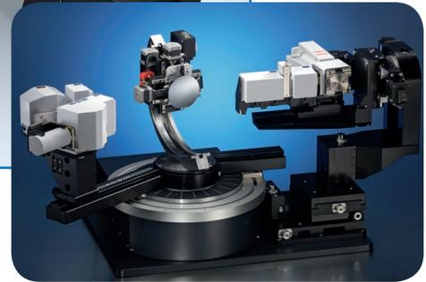
Analyzing epitaxial thin film samples requires a highly parallel and monochromatic X-ray beam in order to have the required resolution in reciprocal space. This is realized with 2-b or 4-b CC monochromators following the Göbel Mirror. Such HRXRD measurements allow evaluating layer thickness, chemical composition, strain/relaxation, layer mismatch, etc.
