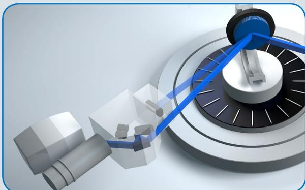
Fig. 6c. High-resolution beam path for XRR on thick films, HRXRD (3-axis geometry) and RSM
