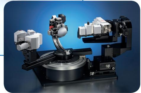
XRR is a surface-sensitive scattering method, which probes variations of the electron density in depth below the surface. Hence XRR can be applied to crystalline and amorphous layers to extract information on thickness, density, surface and interface roughness.
