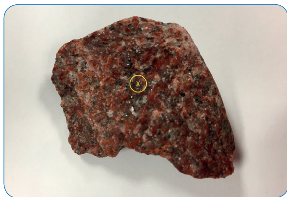
Figure 1. Quartz monzonite rock sample. The yellow X indicates the position where Figure 2a was collected, while the circle indicates the region rastered over resulting in image 2b.
