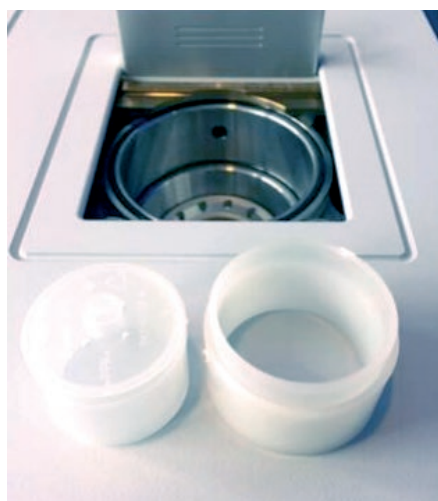
Figure 3: Bruker's dedicated liquid sample cup (Ø 40 mm, left) and the larger SampleCare cup (Ø 51 mm, right)
