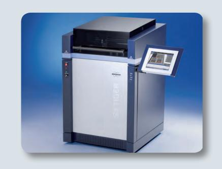
Multielement analysis from Beryllium to Uranium in solids and liquids by sequential wavelength dispersive X-ray fluorescence analysis (WDXRF)
