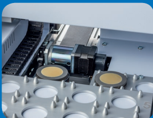
Integrated sample flipper enables careful sample transportation on conveyer belt
