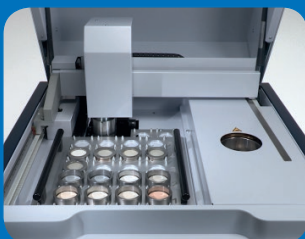
Insertion of sample into sample chamber directly or via buffer positions
