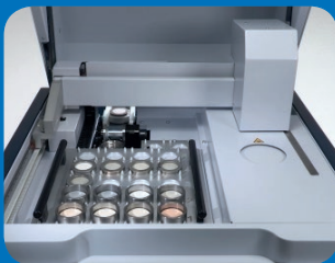
Sample transportation into the instrument from conveyer belt or robot arm
