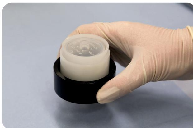
Figure 3: A preparation tool (black) is supplied for failsafe preparation of liquid cup
