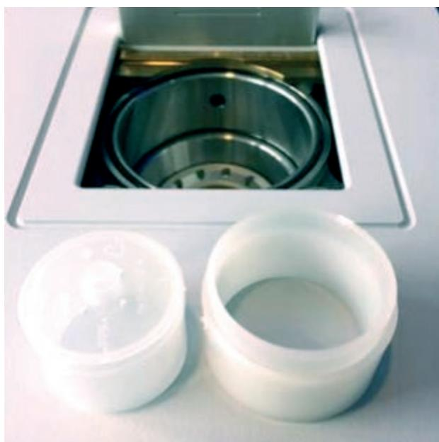
Figure 2: Liquid sample cup (Ø 40 mm, left) and larger SampleCare cup (Ø 51 mm, right)
