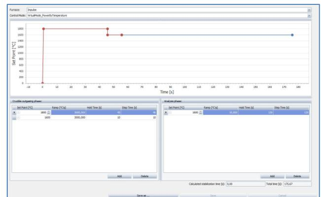
Fig. 1: Electrode furnace programming for OH in copper in FUSION.ELEMENTS. Red: outgassing and delay; blue: analysis time.
