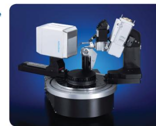
D8 QUEST with Mo sealed X-ray source and TRIUMPH monochromator
